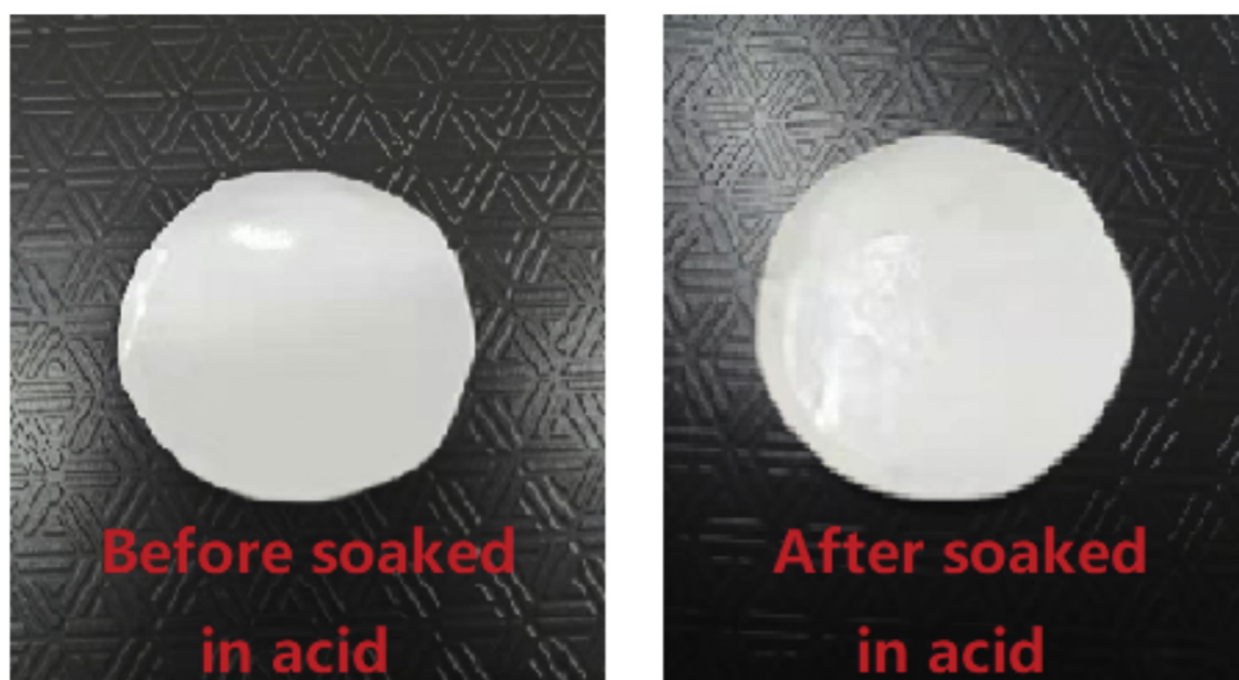
Fig. 8 – Surface images of the membrane before and after it was soaked in acid.
